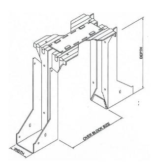
A comprehensive range of single piece non-welded timber to masonry hangers, designed to support timber joists from brick or block walls. As standard all hangers are manufactured from 2.0mm thick pre-galvanised steel to BS EN 10346: 2009, DX51D + G600 compliant with BS6178: Part 1:1990 and to the requirements of BS5268.
